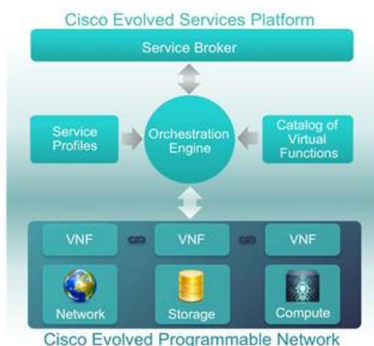
**Figure 12: Cisco Evolved Services Platform Elements [CiscoESP]**
