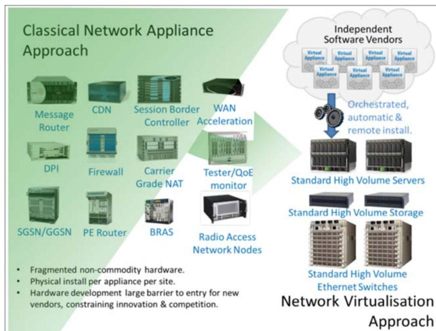
Figure 1: ETSI-NFV-Approach - Vision for Network Functions Virtualisation
