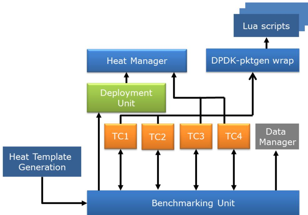
**Figure 4-1: Architectural components of the VNF Characterisation framework**
