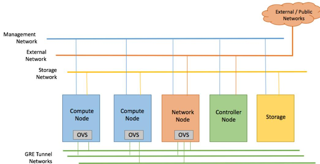
**Figure 2-2: Neutron with GRE segmentation**
