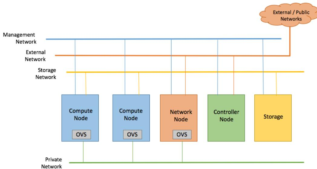
**Figure 2-1: Neutron with VLAN segmentation**
