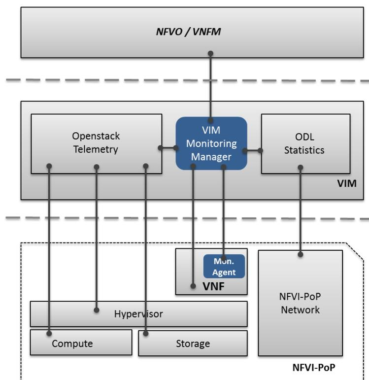
**Figure 2-4. The components of the VIM Monitoring Framework**
