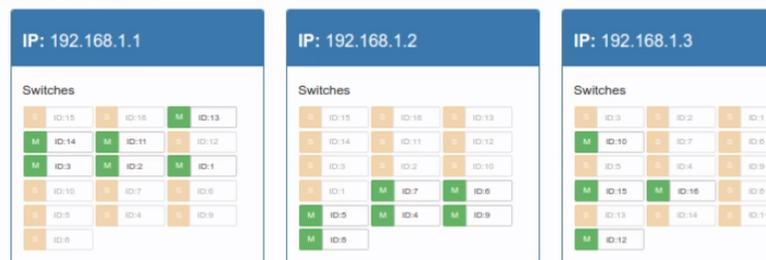
Figure 4-27 Load Balancer Web GUI (after balancing)
