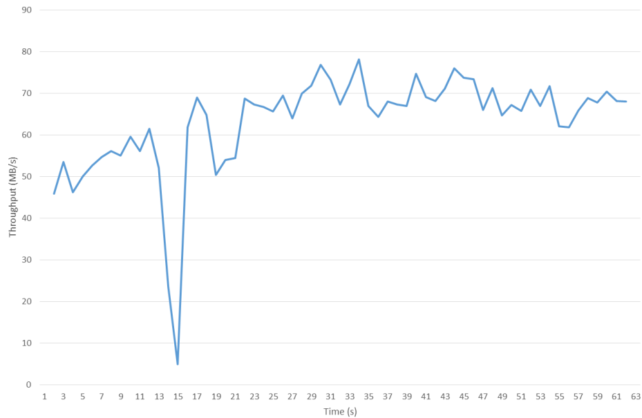
Figure 5-9: Disk I/O: Live Migration with block storage volumes while cache reading
