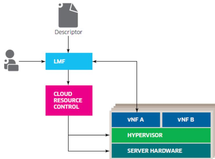
**Figure 10. VNF deployment sequence**
