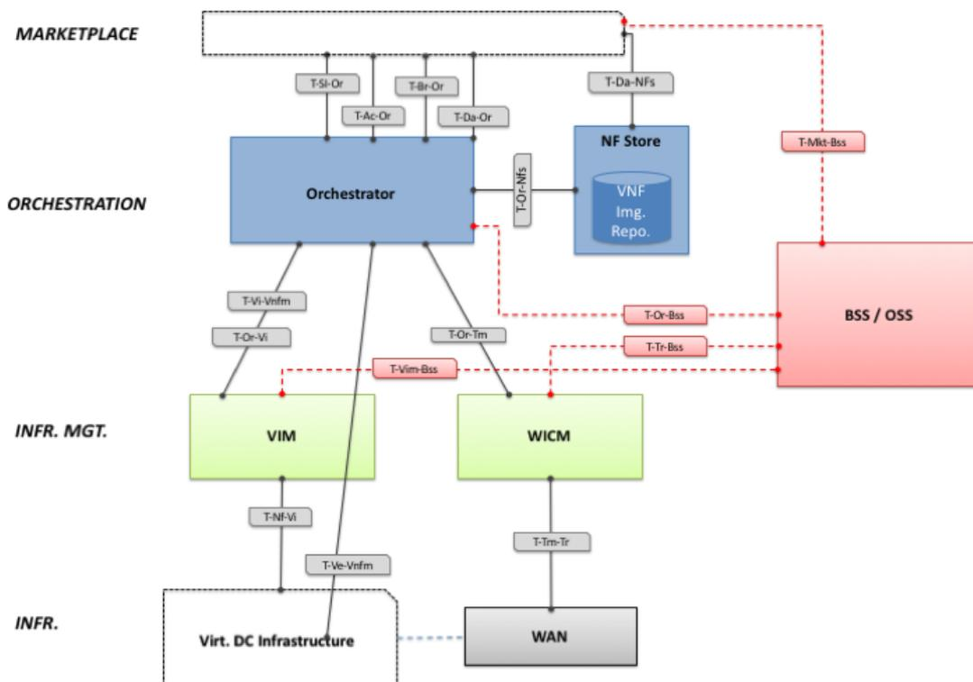
Figure 39. Architecture extension for interfacing with BSS/OSS
