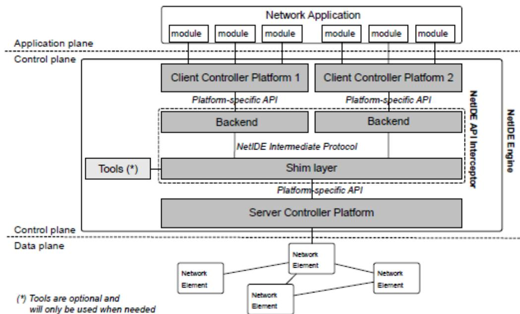
**Figure 18. NetIDE Network Engine Architecture**
