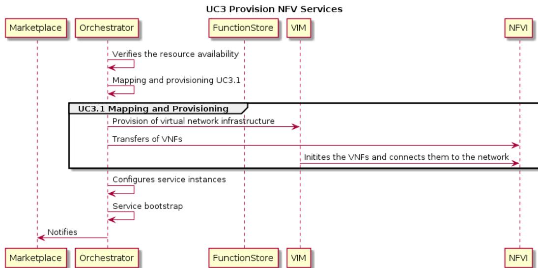
**Figure 30 UC3 Provision of NfV Services Sequence Diagram**
